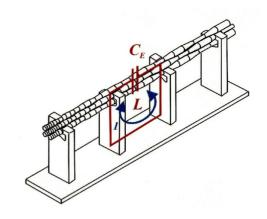
Figure 4: Basic cell of the 4-rod RFQ structure.
