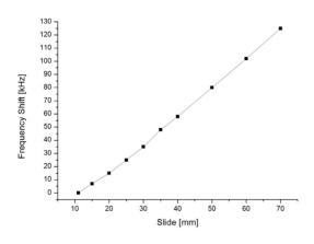
Figure 6: Frequency range of the tuners.
